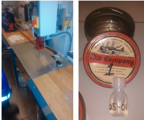
(a) Band saw and core ready to be cut. (b) Tobacco can and flask used to melt and store samples.
